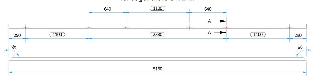
+ = Bohrung Ø 14 mm
